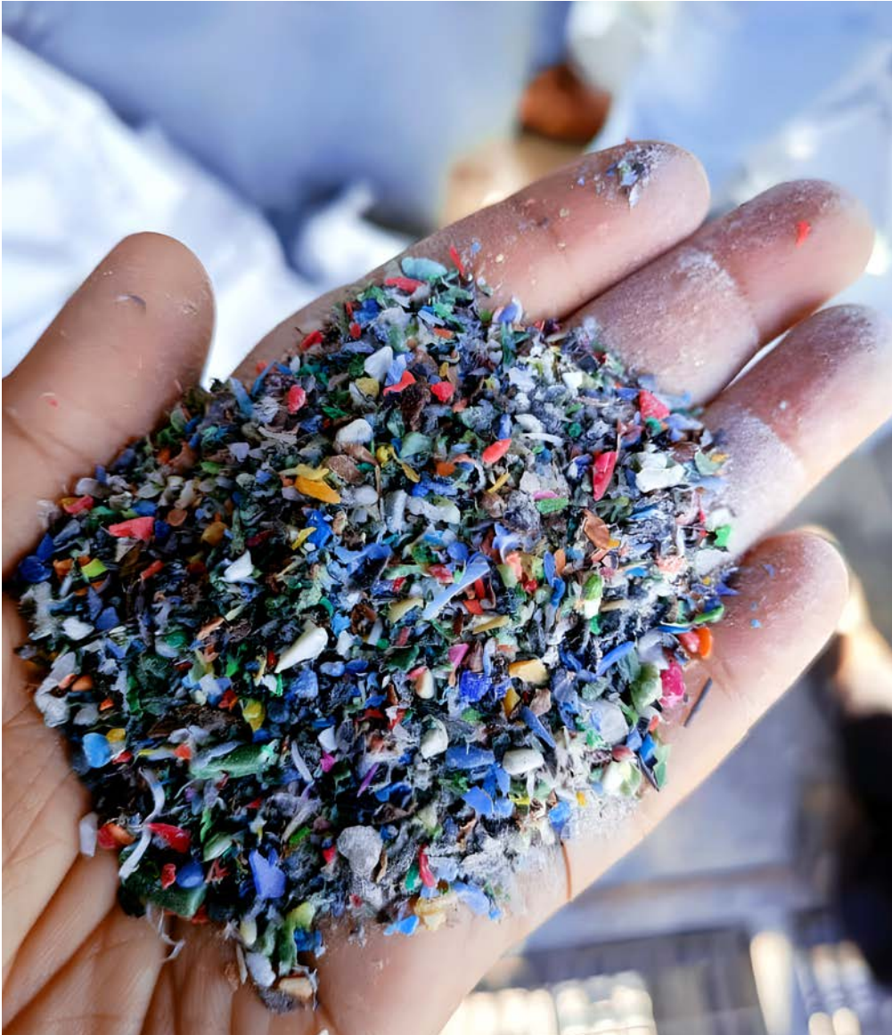
➔ Plastic waste materials used as a binder extender in asphalt mixtures.
