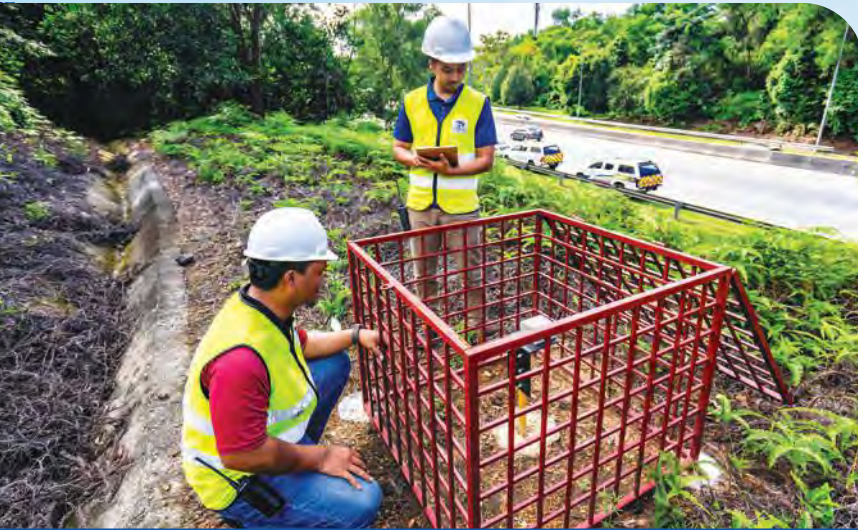
The intelligent high-precision Smart Slope Monitoring System accurately detects slope movements by analysing data from an advanced network of sensors. This comprehensive system includes rain gauges to measure meteorological variables, ensuring precise and reliable slope monitoring.
